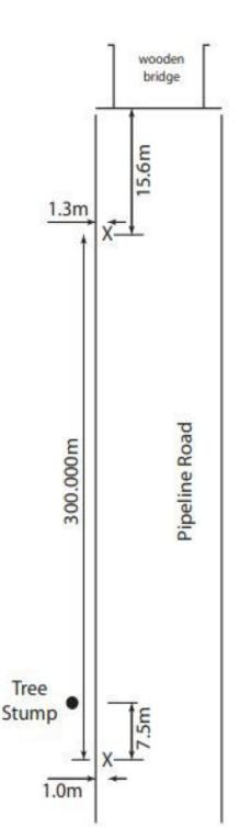
The south pin is located about 15.6m north of the north edge of the wooden bridge on Pipeline road (ie from the edge of the wood). It is 1.3m from the edge of the pavement.
